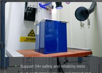
such as thermal runaway, nail impact and drop test
